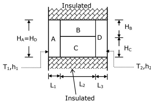
The dimensions are:  $H_A = H_D = 3\text{m}$ ,  $H_B = H_C = 1.5\text{m}$ ,  $L_1 = L_3 = 0.05\text{m}$ ,  $L_2 = 0.1\text{m}$
